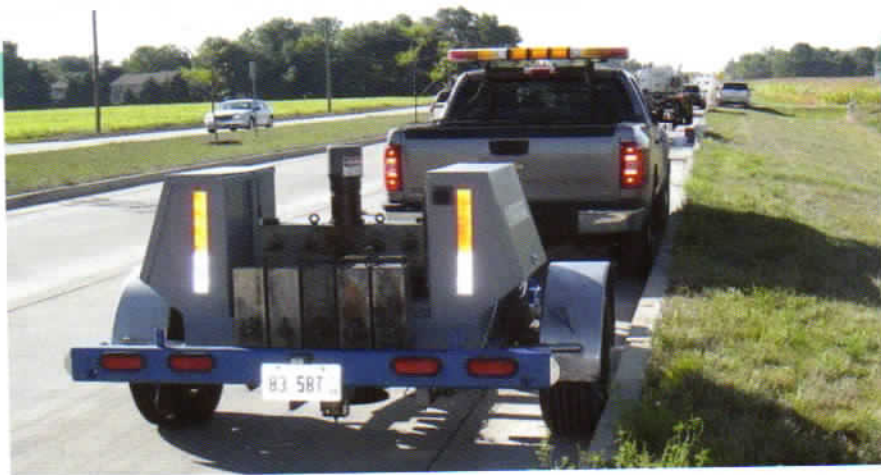
Falling weight deflectometer (FWD) testing important part of field evaluations
