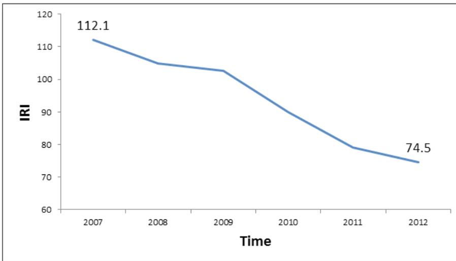
**Fig 1:** IRI measurements for Kentucky's interstate concrete pavements improved from an average of 112.1 in/mile to an average of 74.5 in/mile – the longest sustained improvement in the state's IRI and their lowest recorded average IRI ever.
