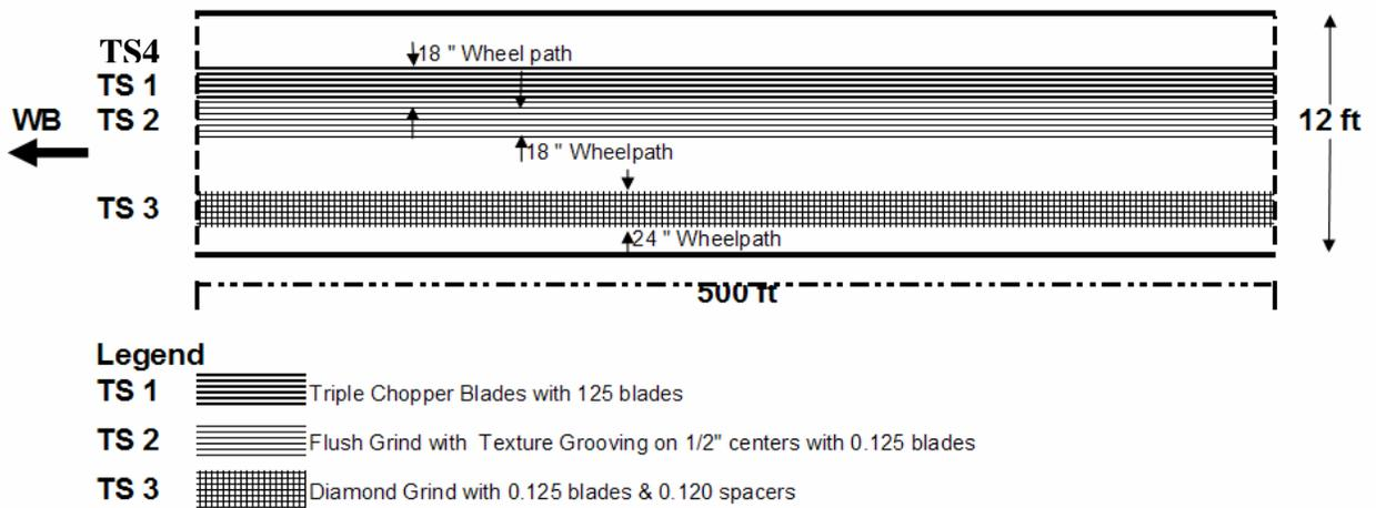
Figure 4 Joint Effect Wheel Track Test Locations
