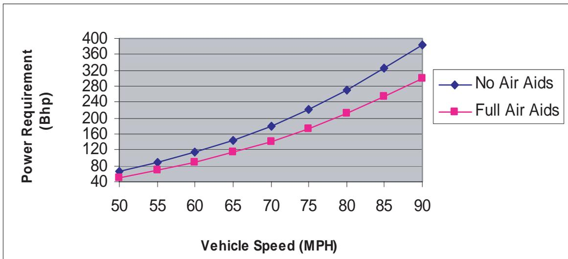
At approximately 0.3 lb./BhpHr fuel consumption, a reduction of 32 Bhp required to cruise at 65 mph results in a savings of about 9.6 lbs. of fuel every hour ( $0.3 \times 32 = 9.6$ ). Since diesel fuel weighs about 7.1 lb./gal., this amounts to a savings of 1.35 gallons of fuel saved every hour ( $9.6/7.1 = 1.35$ ). For a truck running 10 hours per day, that's 13.5 gallons of fuel saved per day. At \$2.45 per gallon of fuel, the dollar savings is \$33.12 per truck per day.
