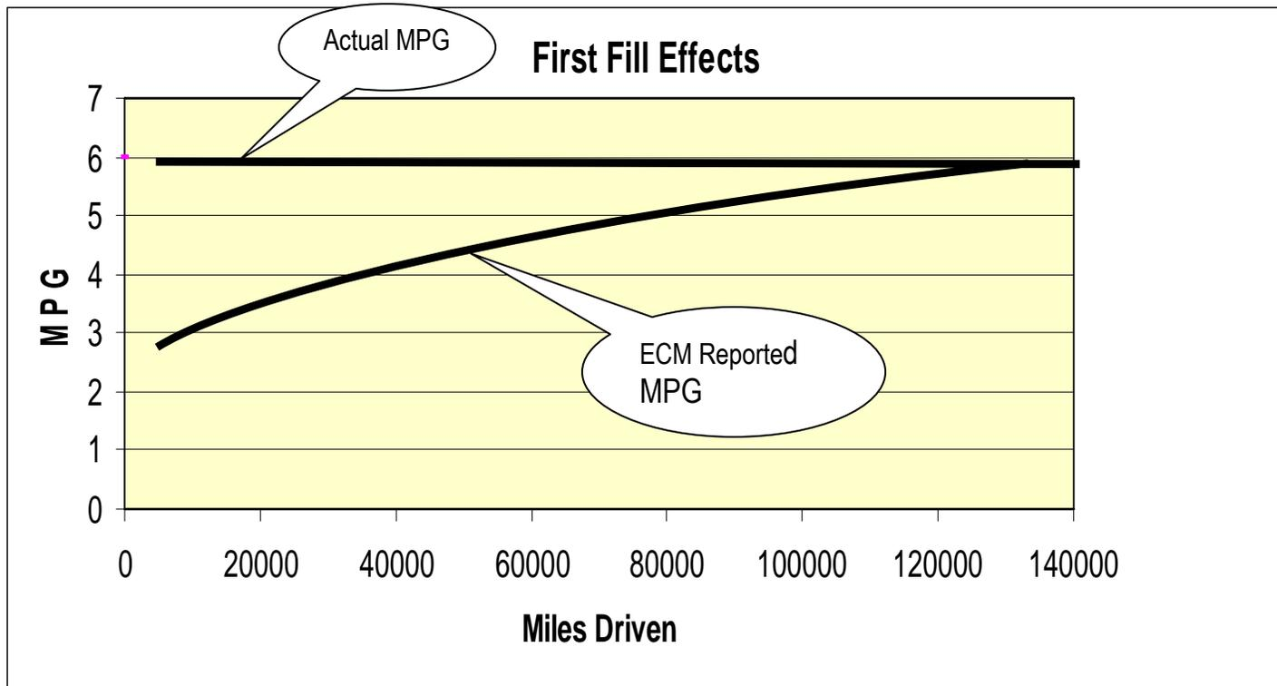
The truck has to run over 145,000 miles before the fuel ticket MPG will match the actual MPG of the truck.
