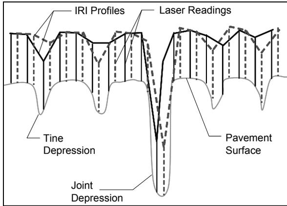
Figure 5. Difference in surface readings due to different laser startup
