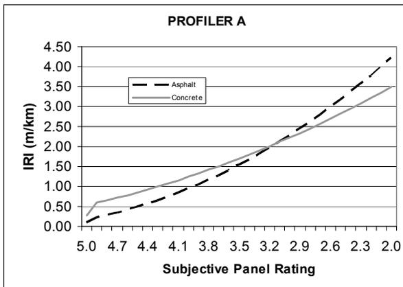
Figure 3. Bias of Profiler A; IRI vs. Panel Rating
