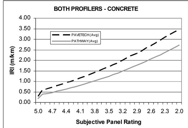
Figure 6. Difference between two profilers on same test section, after calibration
