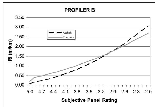
Figure 4. Bias of Profiler B; IRI vs. Panel Rating
