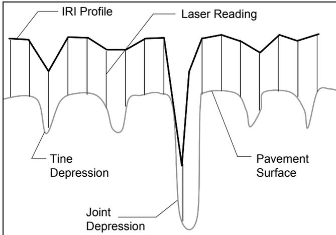
Figure 2. Effect of surface texture and joints on elevation readings of laser
