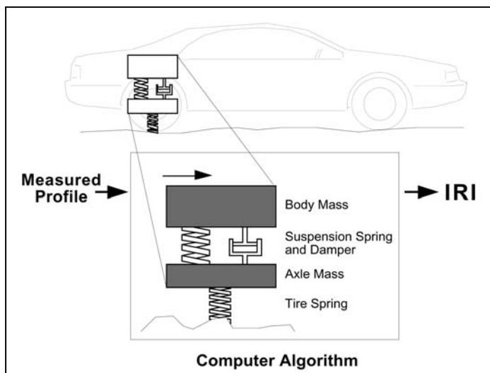
Figure 1. Quarter-car simulation of road roughness
