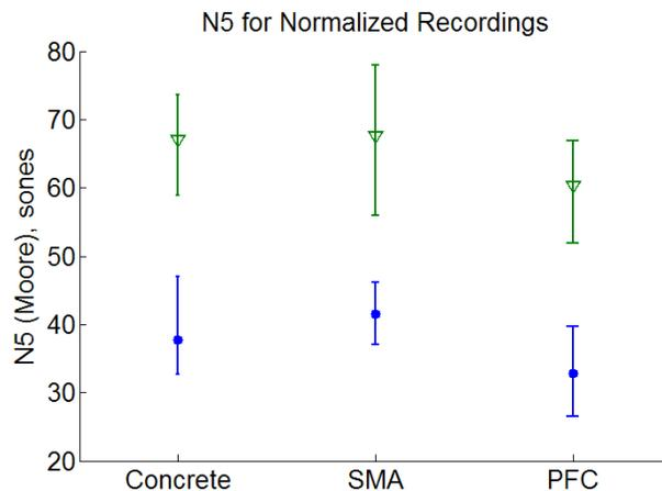
**Figure 6:**  $N_5$  levels for recordings normalized to the same speed based on a 0.2dB /mph increase model. Green lines are for normalized truck recordings and blue lines are for normalized car recordings.
