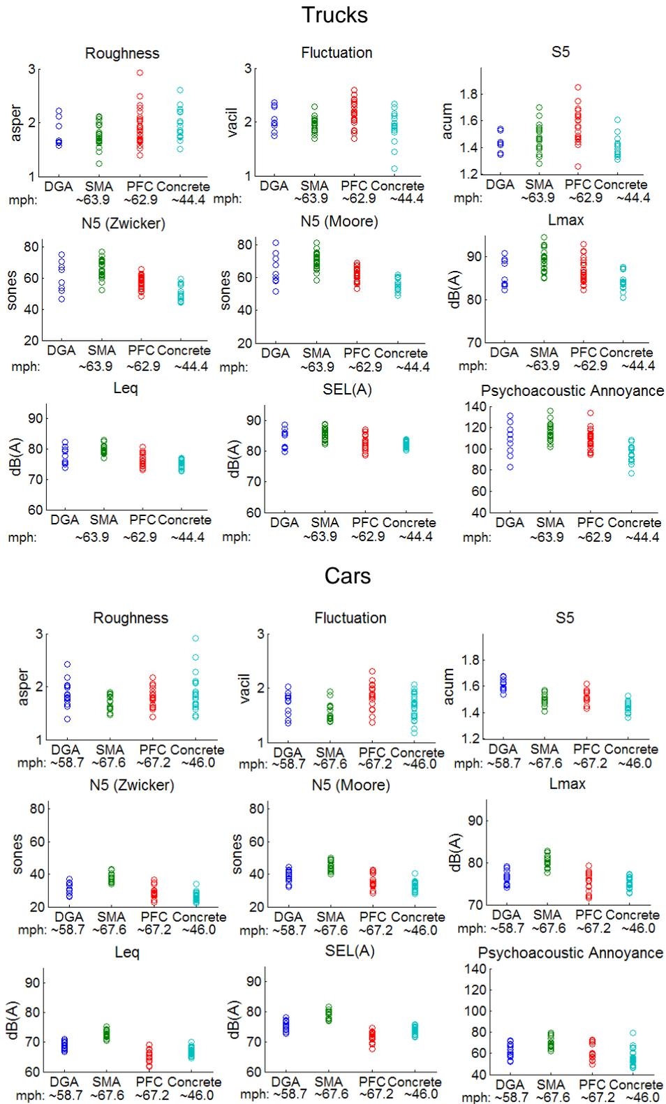
**Figure 4:** Noise metrics for individual truck and car pass-by events. Average speed of vehicles on each surface is indicated on the horizontal axes. The lower levels for passbys on concrete are probably due to the lower speed of the vehicles.
