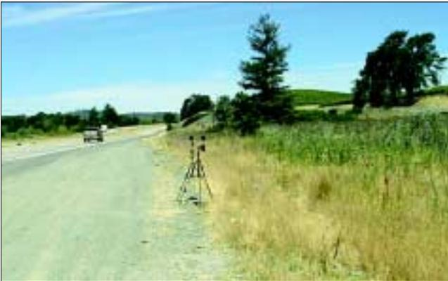
Figure 7. Microphone at 7 m, looking north (diamond grind Site 2).
