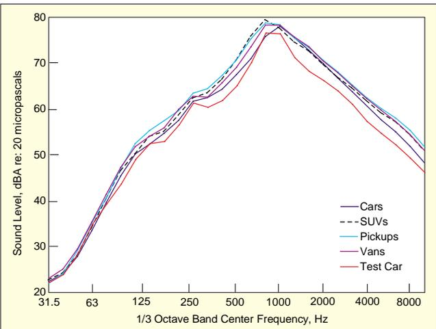
Figure 8. Average A-weighted spectrum of vehicle passbys on longitudinal grooved pavement at 7.5 m.
